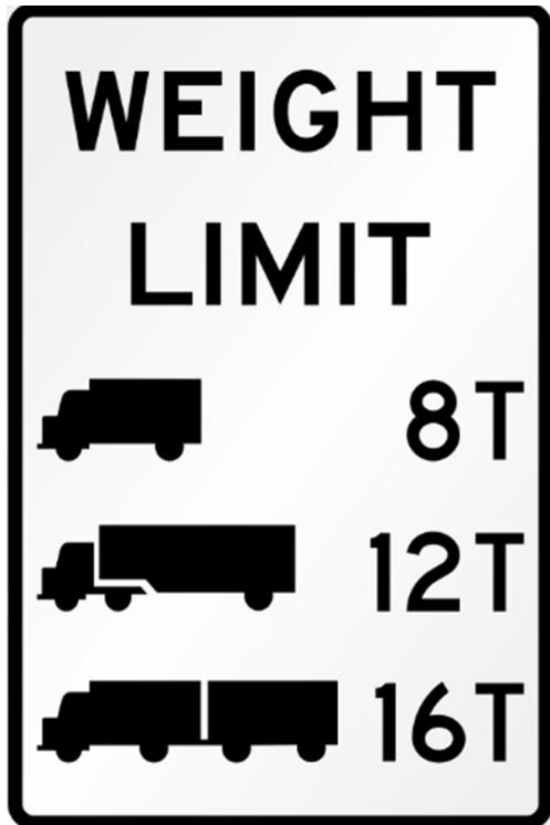
The weight limit of a STRAIGHT TRUCK regardless of the number of axles
