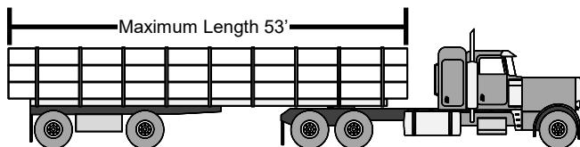
Maximum overall length semitrailer 53' (including load, excluding truck-tractor)
