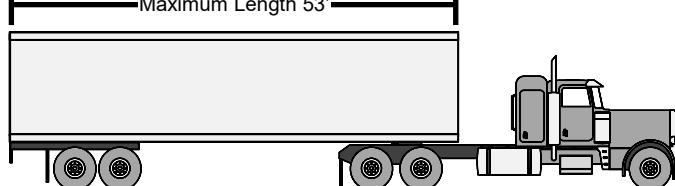
Maximum overall length semitrailer 53' (including load, excluding truck-tractor)
