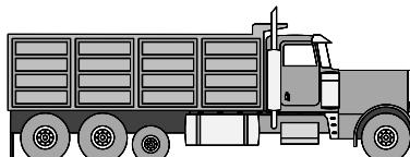
A single vehicle must be registered for the empty weight plus the maximum load to be carried thereon at any one time, for example, 48,000 lbs. (24 ton) farm plate
