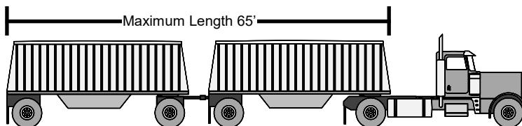
Maximum overall length semitrailer and trailer 65' (including load and connecting devices, excluding truck-tractor)
